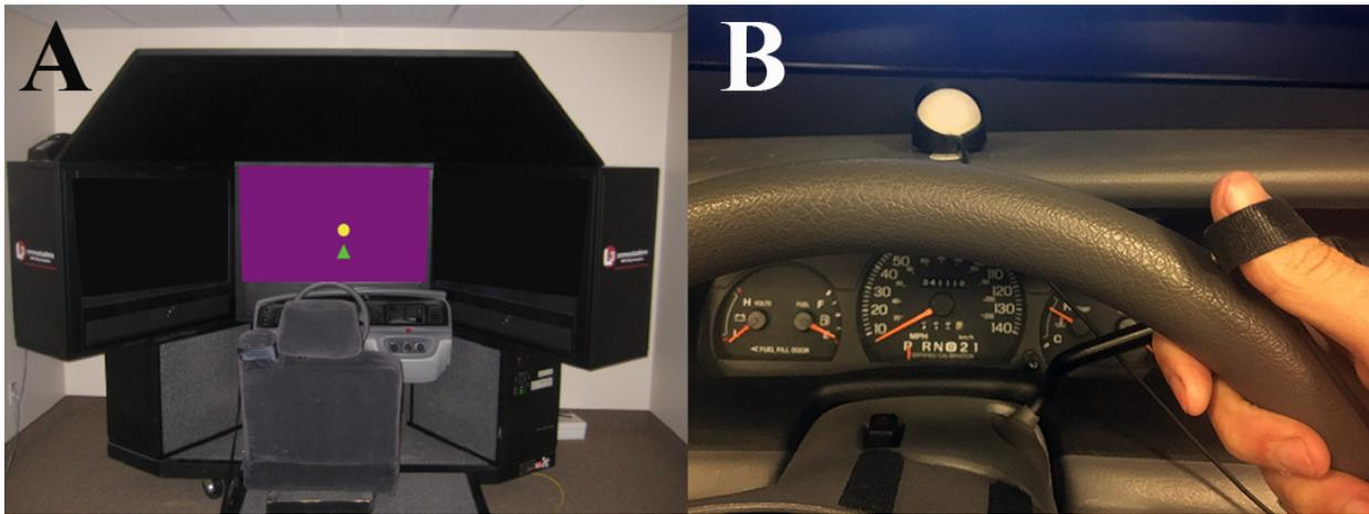
*Figure 2.* Photograph A shows the simulator used to display the pursuit-tracking task utilizing the steering wheel and center screen. Participants control the triangle in an attempt to keep its lateral position equivalent to the circle's lateral position. Photograph B shows the dash-mounted DRT for displaying the dim and bright simple DRT, and choice DRT, stimuli.
