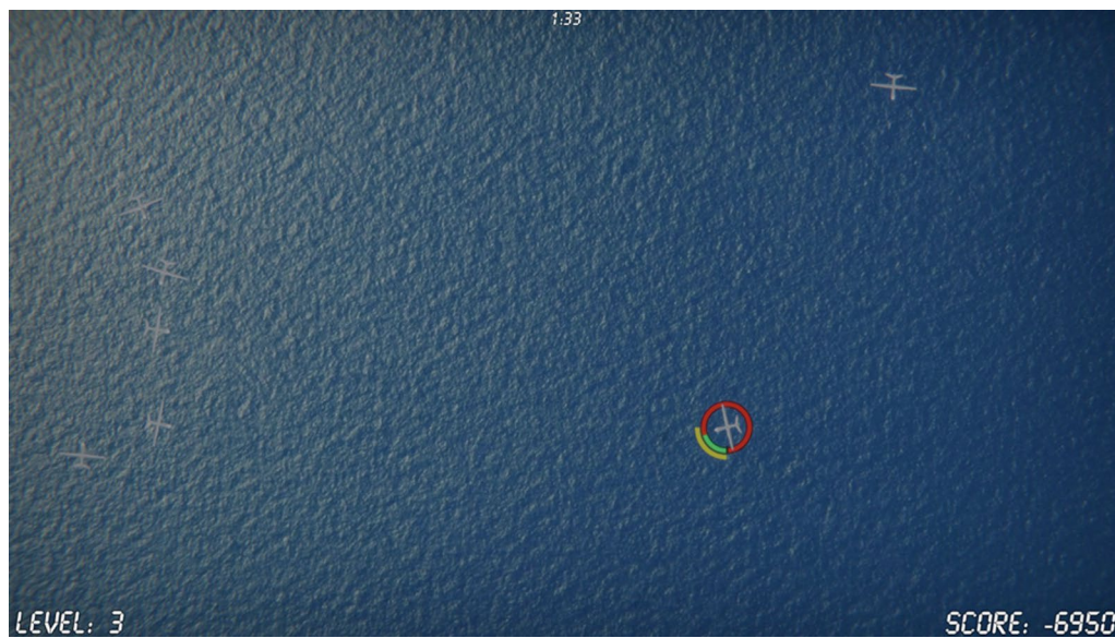
Fig. 1 Task display with seven UAVs. Hovering the mouse over a UAV displays the fuel gauge which shows that the fuel level (yellow bar) is not yet in the green region where it can be refueled. The time remaining in the block is displayed at the top, the difficulty at the bottom left, and the score at the bottom right of the screen
